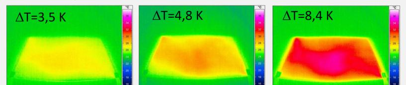
CF-network+ CNT- PU coating, distance of electrodes: 20 cm
