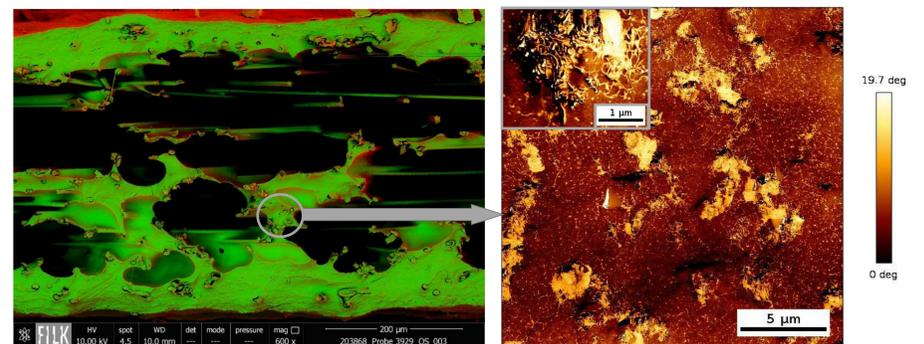
Fig 2: cross section CF network and CF synergist; left: SEM image; right: AFM-image (phase image)
