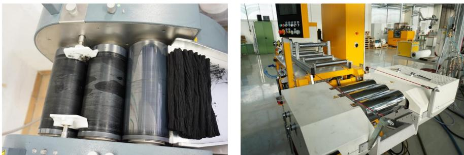
Fig 2: left picture - incorporation of MWCNTs in a silicone matrix on a 3-roll mill
